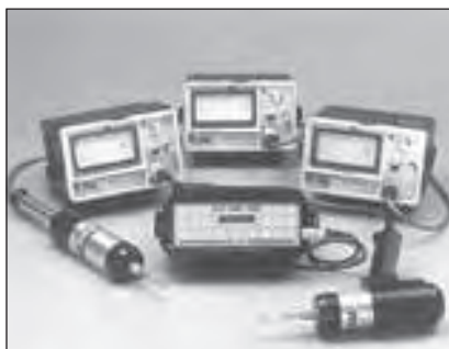
CPI offers both 10.2 eV and 11.7 eV large outline PID lamps for hnu® PI101 Photoionizers.
