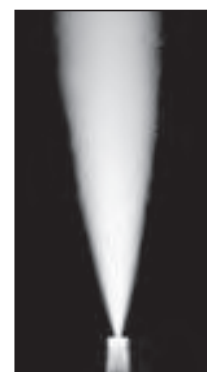
The CPI PFA Micro-Flow Nebulizer produces a fine aerosol for high transport efficiency and high sensitivity.
