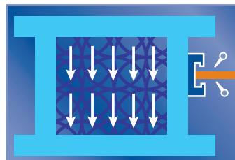
**Packing valve is retracted flush with the wall eliminating dead volume in column.**
