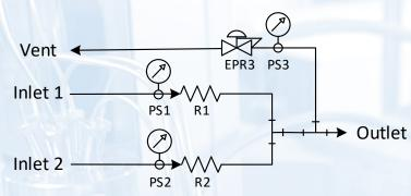
This is our entry level version. In this version, only the outlet pressure is internally controlled by the outlet bypass pressure regulator.
