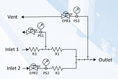
This version has been designed for sample gas containing reactive gases such as sulfurs.
