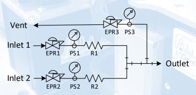
With this version, both inlet 1 and 2 pressures are internally controlled by inline pressure controllers. This version is suitable for most applications ranging from ppb to % impurity level dilution.
