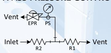
Bypass pressure control is ideal for ultra-trace level dilution and to preserve sample integrity as the valve and pressure sensor are not in contact with the gas used for the dilution. They are located in the bypass vent.
