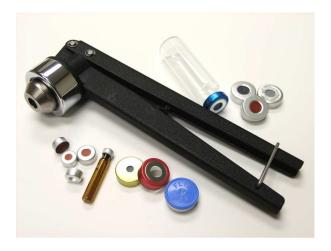
The **Adjustable Crimper** has an adjustment feature which will allow it to be used with a variety of septa, discs, stoppers or liners with a thickness range of 0.25 to 3.0mm. The unit looks like the standard hand crimper but it is supplied with a wrench and special instructions for making adjustments.
