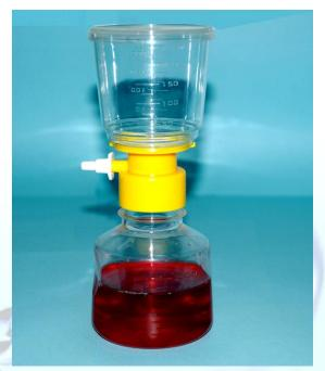
Available in three styles: complete filter/storage unit and bottle top filters and the Reservoir bottle.
