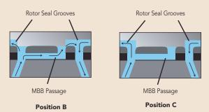
To maintain a constant, desired high-pressure flow, Rheodyne's Make-Before-Break (MBB®) design creates continuous flow between the LOAD and INJECT positions that virtually eliminates pressure transient shock to the system. A passage in the stator face makes a new connection before old connections break. The MBB design — an improvement over bypass-style injectors — does not dilute the sample and is easy to maintain and troubleshoot.
