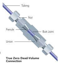
with True ZDV Unions to assist with assembly. With the gauge plug inserted into one side of the union, a hard stop is created for the tubing to bottom out against as it is connected to the opposite port. The gauge plug is removed and then the second piece of tubing is connected, using the first piece of tubing to bottom out against resulting in the two tubes joined together in the center of the union.
