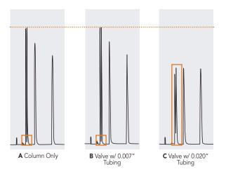
Conclusion: These sequential chromatograms show the effect of adding volume to the flow path through the addition of components.
