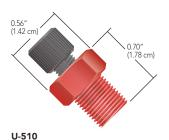
1/8" NPT to 1/4-28 Flat-Bottom Female Adapter for 1/8" OD tubing Includes (1) XP-308 Fitting
