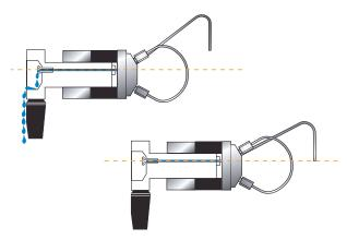
Figure 2 Needle port level compared to the level of vent line outlet: (A) siphoning occurs when the vent line outlet is above the needle port level (B) siphoning does not occur if the vent line outlet is the same horizontal level as the needle port
