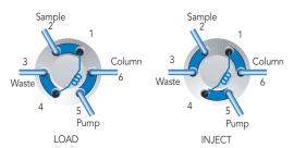
Flow path of Two-Position, Six-Port Injection Valve
