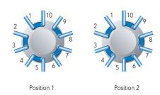
Flow path of Two-Position, Ten-Port Switching Valve
