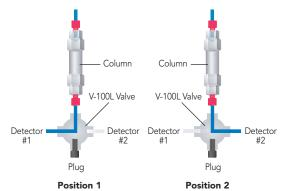
➤ Your detector switching application may require the flexibility of routing the column effluent to both detectors simultaneously while retaining the ability to isolate each detector. Use our 3-Way Flow Switching Valve ("T"), plugging off the fourth port with the included plug (see right).
