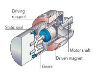
The two magnets couple automatically such that the driving magnet turns the driven magnet and gears without physical contact.
