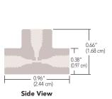
P-170 PEEK 7-Port Manifold 0.020" thru-holes with F-331 Fittings
