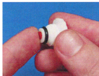
FIG. 6 INSERTING NEW SEPTUM
