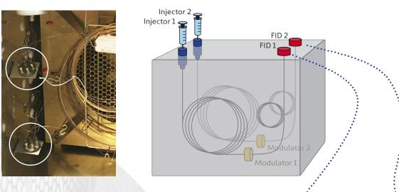
Use of two INSIGHT modulators in a dual-channel configuration immediately doubles productivity, resulting in a swift return on investment. This is illustrated for environmental monitoring of total petroleum hydrocarbons (TPH) using the 'stencil' feature in SepSolve's ChromSpace software.
