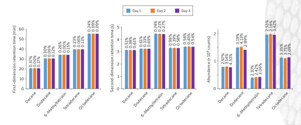
Excellent repeatability of retention times is aided by the use of a dedicated EPC for each column. The charts show <1% RSDs for first-dimension and second-dimension retention times, and <5% RSDs for peak abundance, for 24 injections of diesel over 3 days (n = 8 injections/day).
