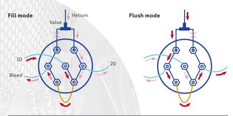
INSIGHT uses a two-stage process involving the sample loop (orange) to achieve effective modulation. In fill mode, the primary column eluate enters the sample loop (with any overfill directed to a bleed line), while the modulation valve directs auxiliary carrier gas to the secondary column. The valve then switches, and the contents of the sample loop are flushed rapidly on to the secondary column as a narrow chromatographic band.
