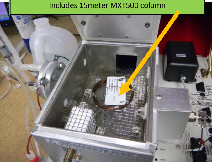
The temperature programmable column oven heats from ambient to 400C.
