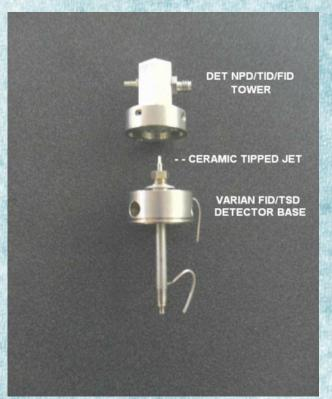
Varian/Bruker GCs – DET tower base and flange designed to custom fit existing FID/TSD base.
