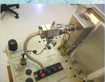
SRI Instruments GC – DET tower attaches to 1/8 inch diameter jet via a Swage fitting. 1/16 inch side Swage port adds Air flow to detector. Custom signal probe arm extends 1.5 inches from tower and bends down in unshielded bare wire.
