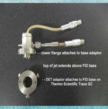
Thermo Trace Ultra GC – custom fits Thermo base. Signal probe terminates in an SMA type connector.
