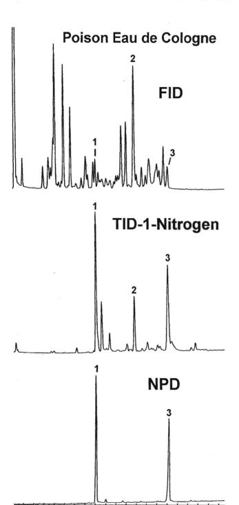
FRAGRANCES. This analysis provides a good example of the selectivity provided by TID-1 and NPD detection versus an FID detector. The sample analyzed was the commercial fragrance, Poison Eau de Cologne (Christian Dior, Paris). Amongst the numerous peaks exhibited in the FID chromatogram, both the TID-1 and NPD detectors selectively responded to just a few of the sample components.
