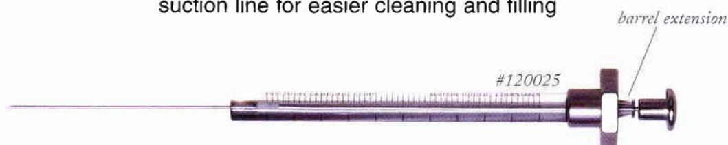
In addition to standard Pressure-Lok features such as PTFE plunger tip and needle seat, the C-120 offers as standard equipment a barrel extension beyond the rear flange which permits attachment of a vacuum bulb or line for easier filling or cleaning.
