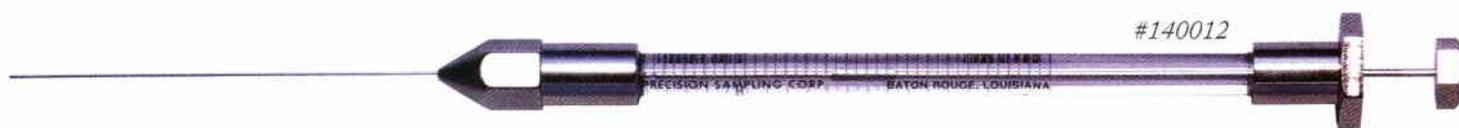
The Series D-140 is designed for small volume injection into gas chromatographs. Since the sample is totally contained within the needle, it is totally displaced by the plunger. Any residual sample or variation in sample size are minimized. (This also means that each size syringe has a different needle design. When ordering extra needles, be careful to specify the correct one.)
