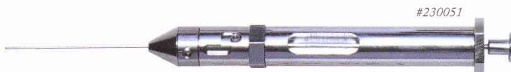
The Micro-Flo high pressure syringe prevents evaporation of lighter components under normal laboratory temperatures at atmospheric pressure. The syringe is encased in metal, with positive PTFE seals and positive plunger stops. The front end houses a special micro-volume annular needle with less than .05  $\mu$ l dead volume and a positive mechanical valve to seal in volatile materials (up to 500 psi).
