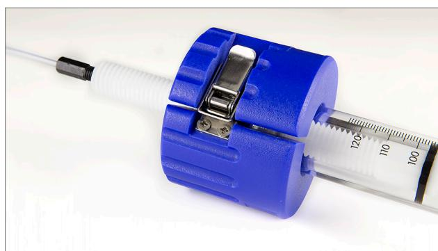
The patented SNAP® closure mechanism provides a safe and reliable means to access the column contents.
