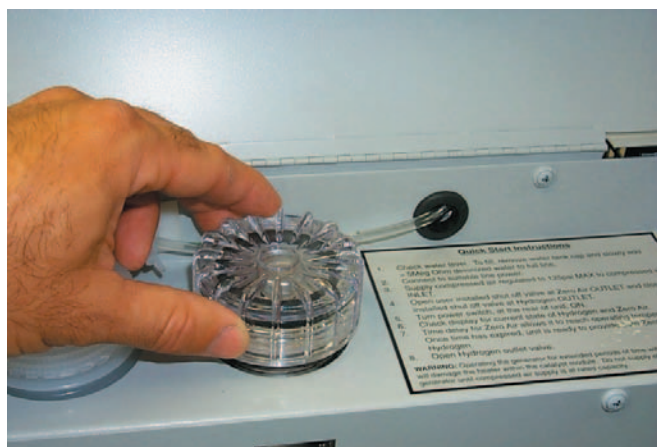
Figure 6 - Unscrew desiccant cap
