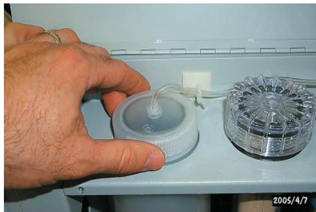
Figure 5 - Screw cap securely on water bottle
