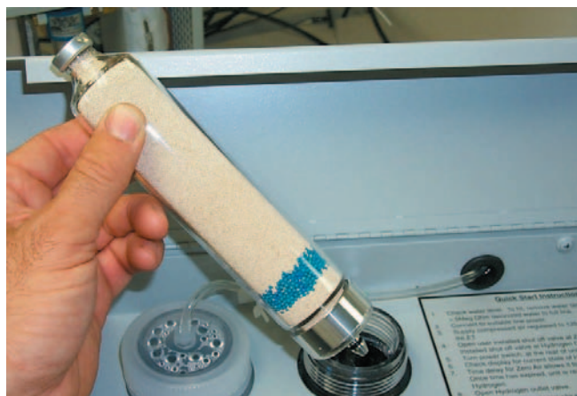
Figure 7 - Insert new desiccant cartridge
