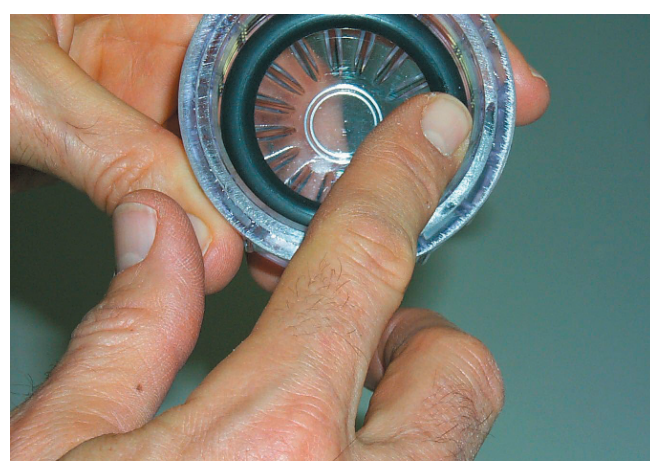
Figure 9 - Make sure the o-ring is centered in the cap before replacing it
