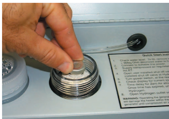
Figure 8 - Press down firmly on desiccant to seat o-ring
