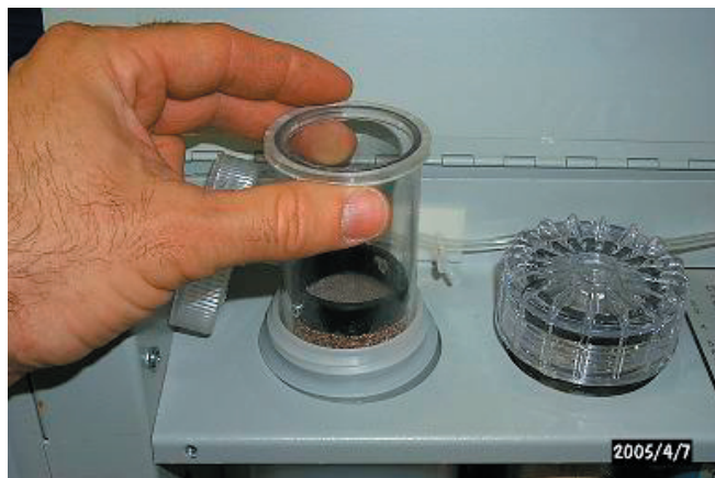
Figure 4 - Set resin bed in bottle
