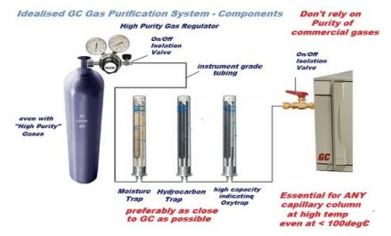
**OXYTraps** are recommended for any GC for all GC type columns to minimise background signals often attributed to bleed even where GC columns are to be operated at high temperatures ( even capillary columns at <100degC)
