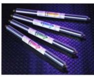
Gas purification is critical to GC performance. Several types of contaminants are detrimental - notably moisture, hydrocarbons, and oxygen. VICI Metronics gas purifier modules are designed to be placed in-line with the GC carrier or detector gas supply to remove these contaminants from the analytical gases prior to their entering the GC.
