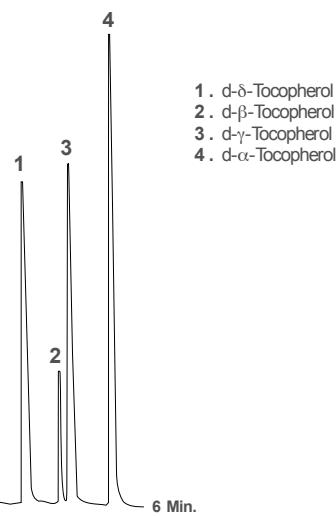
Column: Heliflex AT®-35+, 25m x 0.25mm x 0.20µm
