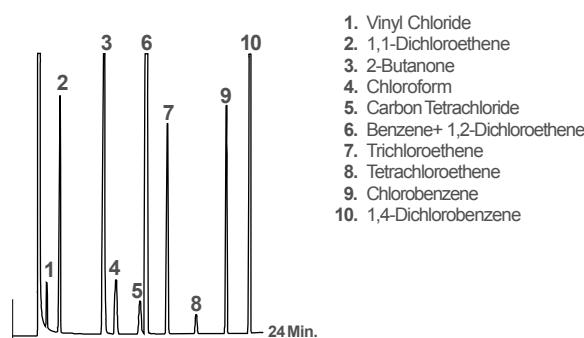
Column: Heliflex AT®-502.2+, 30m x 0.53mm x 3.00µm Part No. **M8635577** (Old Ref. 13792)
