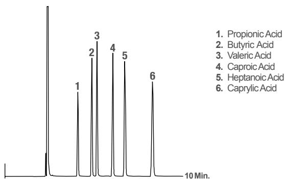
Column: Heliflex AT®-AquaWax DA+, 30m x 0.25mm x 0.25µm Part No. 5122065 (Old Ref. 14537)
