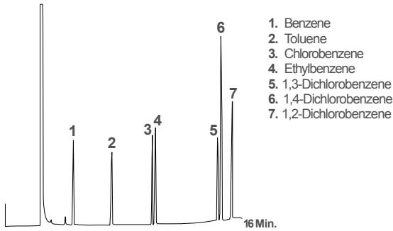
Column: Heliflex AT®-624+, 30m x 0.32mm x 1.80µm
