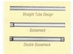
The *straight tube design is* the most common splitless sleeve design. This liner is ideal for low molecular weight samples that are not prone to thermal decomposition. if used for high molecular weight sample analysis, packing material is recommended to aid in sample vaporization. The drawback with using packing material
