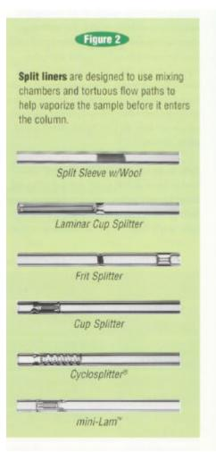
surface area in the cylindrical glass screw also helps to trap non-vaporized sample, therefore making it ideal for dirty samples
