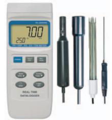
One meter for multi purpose operation: PH/ORP, DO, CD/ TDS Meter • pH: 0 to 14.00pH, ORP: ± 1999mV 🔵 Conductivity: 200 uS/2mS/20 mS/200mS • Dissolved oxygen : 0 to 20.0 mg/L • ATC (automatic temp. compensation) Real time data logger (record year, month, date, hour, minute, second ), 16,000 data logger
