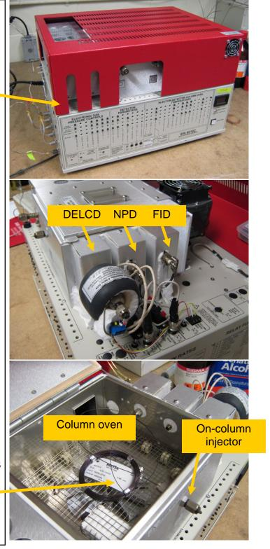
Two additional columns can be connected to the Heated Injector. One of these columns goes to the NPD detector and the other to the DELCD detector. The Heated Injector splits the sample onto the two columns using a two hole ferrule
