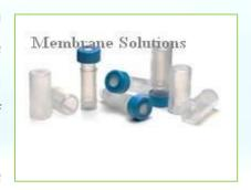
Each unit includes two parts: a chamber and plunger. A filtration membrane on the end of the plunger and pre-attached cap/septum on the other. When using, sample is injected into below chamber, then press the plunger manual, positive pressure forces the filtrate up into the reservoir of the plunge.
