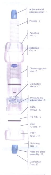
Note: - columns must never be used under gas pressure. This may result in an explosion.
