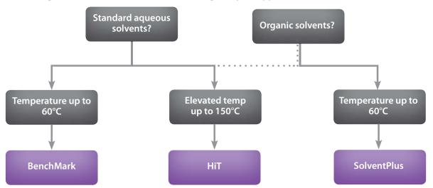
BenchMark columns are designed to suit the majority of standard laboratory chromatography applications. They are ideal for aqueous systems and compatible with solvents used in common liquid chromatography applications such as protein purification.
