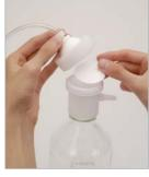
Place membrane filter on top of grid.
