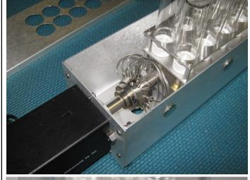
The septum of the vial is punctured by a 27 gage Luer-lok needle when the vial is inserted into the sampler.
