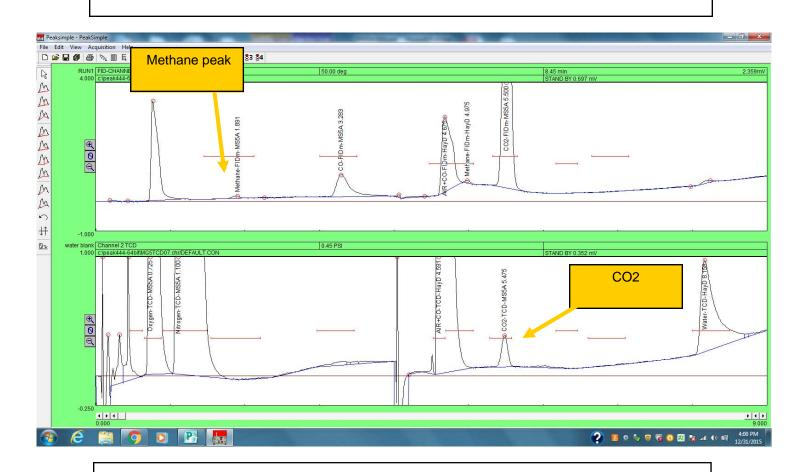
This is room air which has 2ppm of methane, 400ppm of CO2 and 10,000ppm of water.
