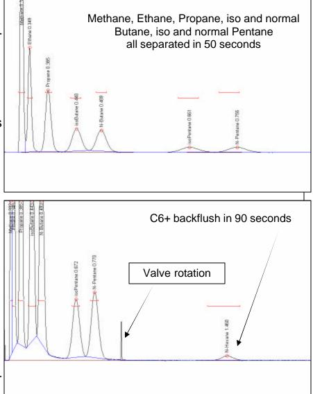
be achieved in about 50 seconds. The SRI 8610C GC was equipped with a 15meter MXT 1 column, an FID detector, and a gas sampling valve plumbed to inject and backflush under control of the included PeakSimple data system. The FID amplifier was set to medium gain and modified to reduce the time constant.
