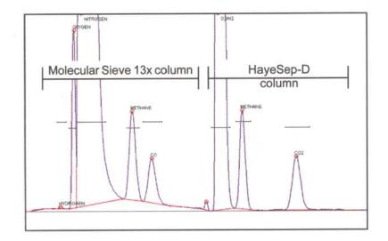
This chromatogram shows the separation of a 1% Gas Standard sample on a MG#2 GC equipped with a TCD detector. The first 5 peaks came off the MoleSieve column, and the following 3 peaks came off the HayeSep-D column. Note that the methane elutes twice, once from each column.
