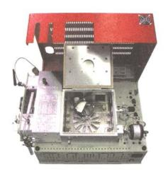
Up to five injectors can be installed on the same GC.
