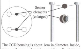
The CCD housing is about 1cm in diameter. Inside, there are 2 sensor elements consisting of a platinum wire embedded in a catalytic ceramic bead.
