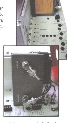
about 1 nanoampere) through the electron cloud, are forced to pulse at a faster rate to compensate for the decreased number of free electrons. The pulse rate is converted to an analog output, which is connected to the data system.
