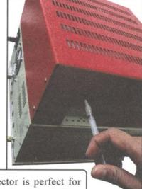
The On-Column Injector is perfect for liquids and gases with high and low boiling analytes. Even very high temperature analyses are easily performed using simple, reproducible on-column injection.
