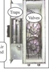
Shown here is a dual TO-14 Air Concentrator with four traps and two gas sampling valves.
