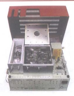
The Greenhouse GC is designed for the detection of carbon dioxide (CO<sub>2</sub>), methane (CH<sub>4</sub>) and nitrous oxide (N<sub>2</sub>O). Depending upon the volume of the sample loop on the gas sampling valve, it can detect trace levels or high concentrations. It may be used for stack or ambient air monitoring, or in a plane for atmospheric air analysis. The chromatogram at left was generated by a Greenhouse GC with a 5mL sample loop.
