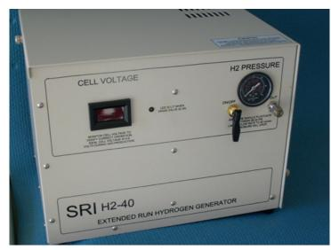
The H2-40 produces 40 milliliters per minute of hydrogen gas at 30 psi. using deionized water, or even readily available distilled water from grocery and convenience stores. The H2-40 can supply enough hydrogen gas for one FID detector, in addition to providing the GC carrier gas. During operation, it also stores enough hydrogen to operate a split injector for very short periods.
