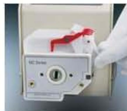
B. After that, the cartridge can be taken out lightly.
