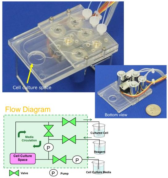
This all-in-one system on a disposable PDMS chip is a microfluidic module designed for cell culture. It has peristaltic pumps, miniature valves, and a built-in cell culture space which can be observed under a microscope. The replaceable chip is sterilisable before use. A remote controller using an Android application is available for this module upon request.
