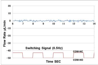
Measurement method: Measure the flow rates at the N.C. ports with a micro flowmeter when turning the valves on/off while filled with water and with the COM. and N.O. ports plugged.
