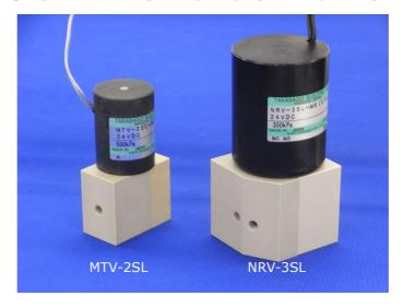
The solenoid-driven slider valve is a kind of shear valve in which a shutter called a "slider" moves vertically and shuts off the flow path. The pumping volume which occurs when a diaphragm valve opens and closes, or the dead volume in which some fluid may stay in the valve is reduced to almost zero, preventing reduction of accuracy in analysis or fluid dispensation. Furthermore, the pressure capability of this slider valve is greatly improved.
