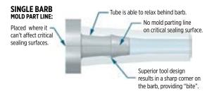
edge on each barb of a molded multi-barb fitting – a feature critical to the performance of the connection.
