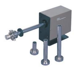
Valves which will be installed in ovens or heated zones require a standoff assembly, which locates the actuator out of the heated zone and supports both the valve and the handle or actuator. The 5/8" outside diameter standoff tube extends through the oven wall and is secured by means of a clamp ring supplied with the assembly.
