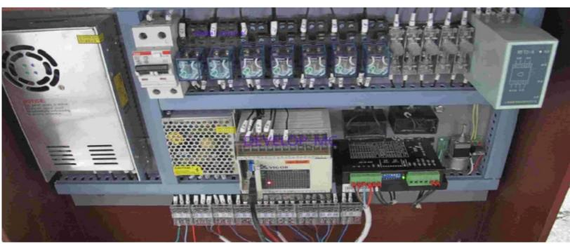
XL-18 Vial Filling Stoppering Capping Machine - PLC Commtrol Wiring Simplicity ? 220VAC to Transformer to 24VAC / DC ?
