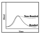
Restek has been able to bond the liquid phases to the solid support using proprietary chemistry
