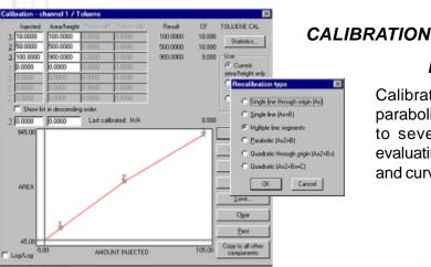
Calibrate peaks six ways (multi-line, quadratic, parabolic, etc.) using single or averaged data at up to seven concentration levels. Statistics for evaluating line fit quality, modification date audit trail, and curve printout help to ensure defensible results.
