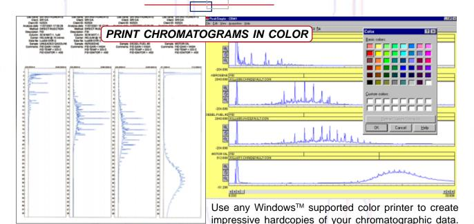
Print multiple chromatograms per page for easy detector-to-detector comparisons and paperwork consolidation. Print overlaid data in contrasting colors with adjustable line weight.
