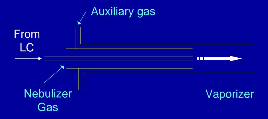
The vaporizer tube temperature is optimized for complete transfer to the vapor state
