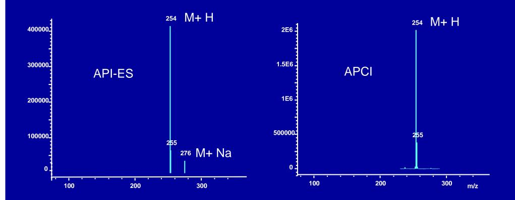
Comparison of the mass spectra typical of Electrospray vs. APCI
