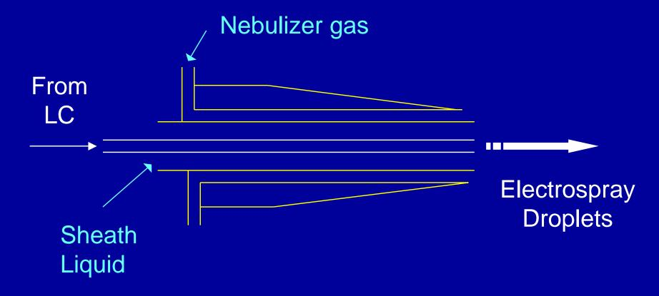
Example of an electrospray needle design (coaxial flow)
