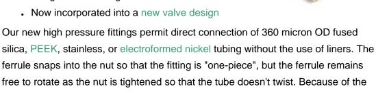
360 µm fittings are dedicated for use with either fused silica, metal, or PEEK tubing; components cannot be mixed or used with a different tubing material.
