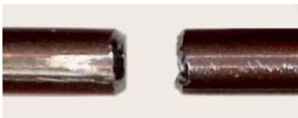
Proper and improper MXT® column cuts.
