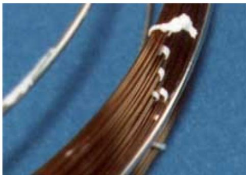
**Do not remove the high-temperature string holding the fused silica capillary column inside the Restek cage.** The high-temperature string is capable of withstanding more than 400°C and does not decompose during continuous operation at oven temperatures used in capillary chromatography.
