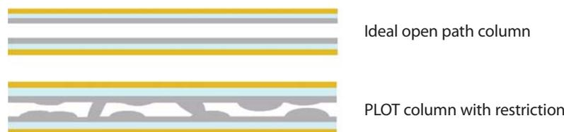
In order to evaluate flow restriction reproducibility, Restek is introducing a new factor: the flow restriction factor (F). This factor is based on the retention time of an unretained marker compound, as measured on both coated and uncoated tubing using the same backpressure setting (Equation 1). For quality control purposes, methane is used as the marker when evaluating porous polymer columns and helium is used for testing Rt®-Msieve 5A columns.
