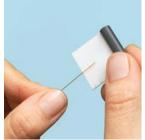
Check the cut against the white of the scoring wafer. Look for a clean, square cut.
