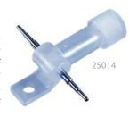
Special geometry at the base of the housing allows bubbles entrained in the inlet fluid stream to rise and be trapped in the reservoir. The gas/liquid interface is easily visible through the translucent wall of the device. Loosening the airtight cap releases the trapped gas. The debubbler is fitted with a bracket and universal connecting tips.
