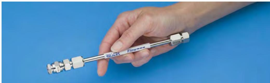
Assembled column with Trident™ integral guard system
