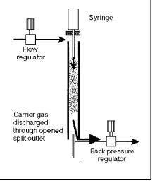
and the column entrance for sample evaporation and mixing across the vaporizing chamber. If the split flow rate is lower, i.e. vapors are formed more rapidly than gas is discharged, a long or a short needle is best suited depending on the carrier gas supply system involved (Fig. 2 or 3).
