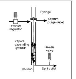
long. The commonly used 5cm needles enter the liner by less than 4cm and merely exploit the upper half of the chamber. 500 ul thus injected already overfill the injector liner, i.e. cause sample material to be expelled through the septum purge outlet or to penetrate the carrier gas supply line.
