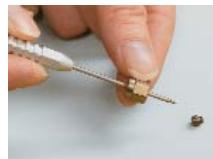
Dislodge a stuck ferrule quickly and easily—with out scoring the fitting.
