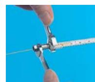
Tighten the assembly with moderate force to ensure a properly seated ferrule. Loosen the assembly and remove the column and column nut with seated ferrule.
