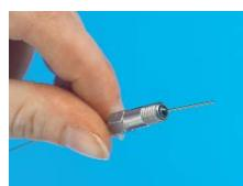
The ferrule will be properly seated in the column nut, and should remain in place when light force is applied. If it slides loosely on the column, repeat procedure.
