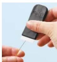
Hold tubing firmly in one hand, allowing about two inches to extend freely. Hold the scoring wafer at a 45° angle to the tubing. Exert slight pressure—just enough to put a slight arc in the tubing. Pull perpendicularly across the tubing.
