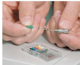
Dislodge ferrules or remove silica deposits with the Jet Reamer/Ferrule Remover.
