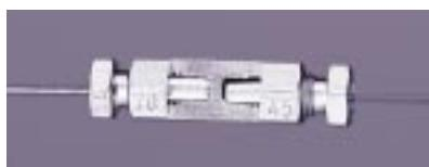
The central component of this connector is a metal-jacketed graphite ferrule. The Gerstel GRAPHPACK® connector can be used for connecting metal capillary columns to fused silica capillary columns.
