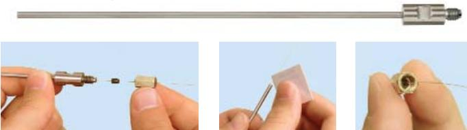
Install the nut and ferrule onto the column, then insert the column through the installation tool, exposing several centimeters at the exit end. Tighten the nut.
