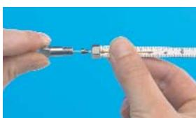
Install the column nut and ferrule onto the capillary column. Cut the column end squarely. Slide the column into the installation gauge to the recommended insertion distance. Finger-tighten the column nut.
