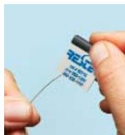
Hold the scoring wafer at a 45° angle to the tubing. Use gentle pressure and a smooth, perpendicular stroke.
