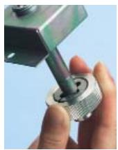
Screw the rethreading tool completely onto the injection port in a clockwise direction. Depending on the severity of thread damage, this may require some force.
