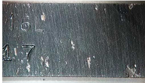
**Table 1** Silcosteel®-CR treated coupons show little weight loss after exposure to 6% w/w ferric chloride solution.
