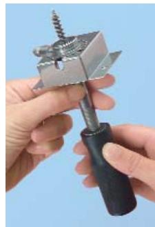
The critical seal at the base of a split/splitless injector allows a seal to form between the injection port and the inlet liner. This critical seal wears over time and may become scratched or pitted, which compromises the sealing ability of the injector. Use the Restek injection port repair tool to easily resurface the inlet seal and remove contaminants; it saves time and money by preventing leaks.
