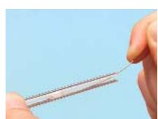
Place a 1cm plug of loosely bound wool in the liner. Adjust its position with the puller/inserter tool.
